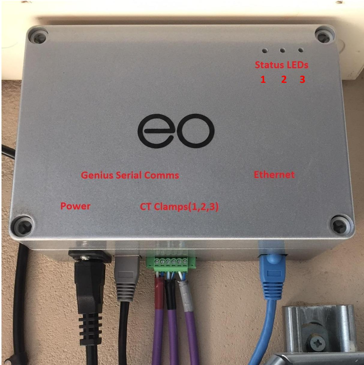
Figure 4 - Connections to the Genius Hub
