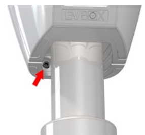
Figure 6: Positioning the hex socket bolts
