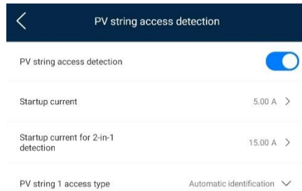
Figure 5-29 PV string access detection
