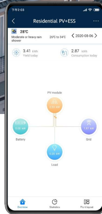
Real-Time Power Flow
