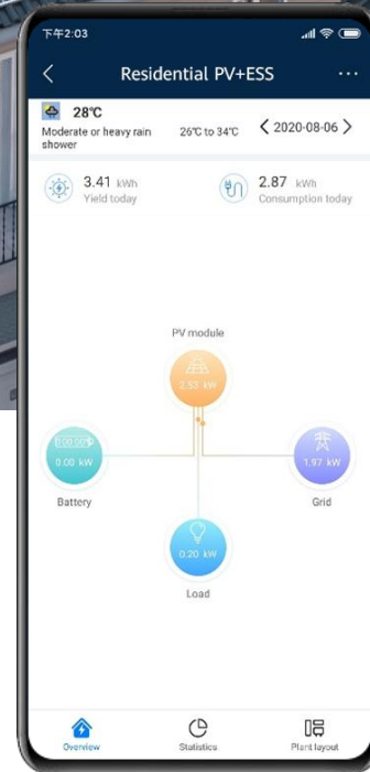
Real-Time Power Flow
