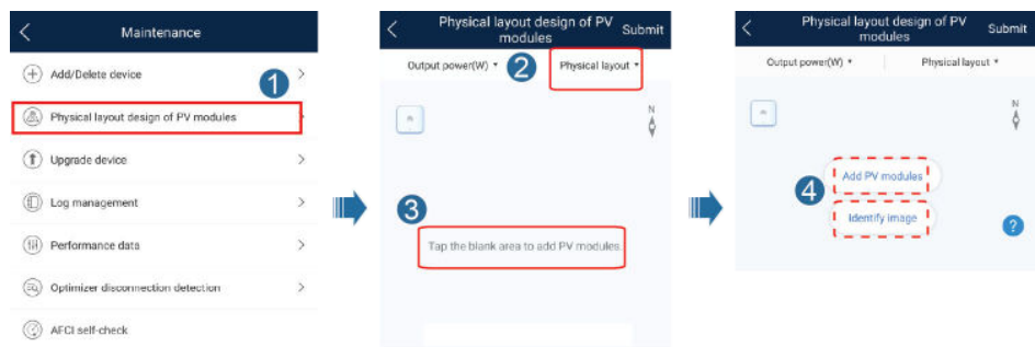
Figure 7-8 Physical layout design of PV modules
