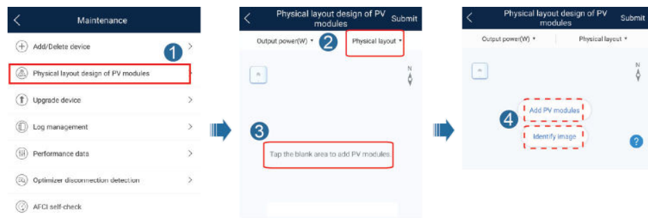
Figure 7-8 Physical layout design of PV modules
