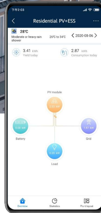
Real-Time Power Flow
