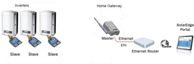
Figure 3: Connection to a Multiple Inverter Wireless Bus
