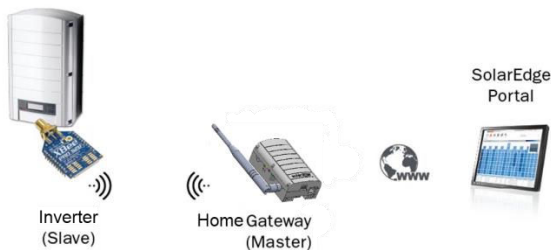
Figure 2: Connection to the SolarEdge Inverter
